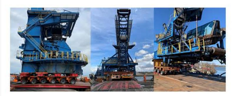
PSC recently utilized our 10-meter drop-deck trailer and a pair of six-line Goldhofer SPMTs to perform a "6-deck-6" over-the-road transport of a new 20' long x 9'6" wide x 16'8" tall transformer weighing 250,000 pounds. The transformer was received at a rail siding and then transported approximately four miles to its final destination where it was offloaded via jack & slide method onto a concrete pad in a live substation.
